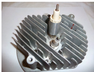
Illustration 7: Screw the Direct Hits onto the spark plug. ** Hand tighten only!! Do not use a tool to tighten the Direct Hits.
