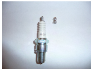
Illustration 5: Remove the nut from the top of the plug if it came with one. Gap to engine mfg specs.
