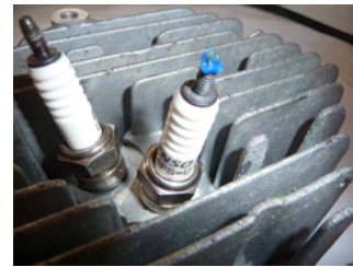
Illustration 6: Install the plug(s) and torque to the mfg. specs. Put a dot of blue Loctite on the top couple of threads.
