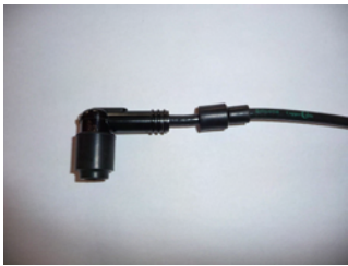
Illustration 4: Screw the cap into the wire. There is a threaded stud inside the cap. Slide the boot on.
