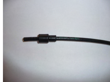
Illustration 3: Slide the weatherproof boot onto the spark plug wire. **Note** Solid rubber caps need no boots
