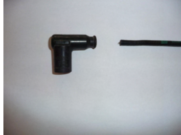
Illustration 2: Remove your existing spark plug cap from the wire
