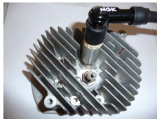
Illustration 8: Snap the new cap on the Direct Hits. Done!!
