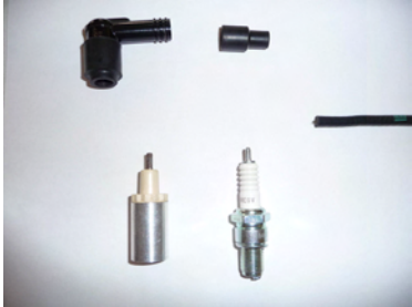
Illustration 1: These are the basic parts for an installation. A Non-resistor plug, the Direct Hits and the new spark plug cap
